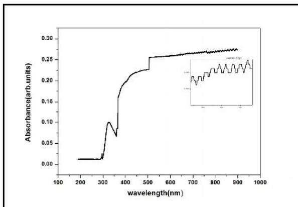
**Fig. 1: Absorption Spectra of Copper nanoparticles**
