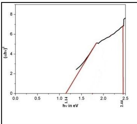
**Fig. 2: Band edges of Copper Nanoparticles**
